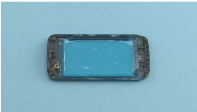
21) Protect also the TOUCH PANEL from the inside with protective film.
