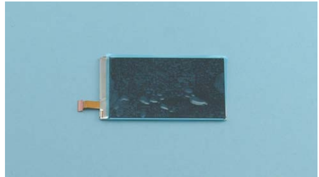
20) Protect the DISPLAY with protective film.
