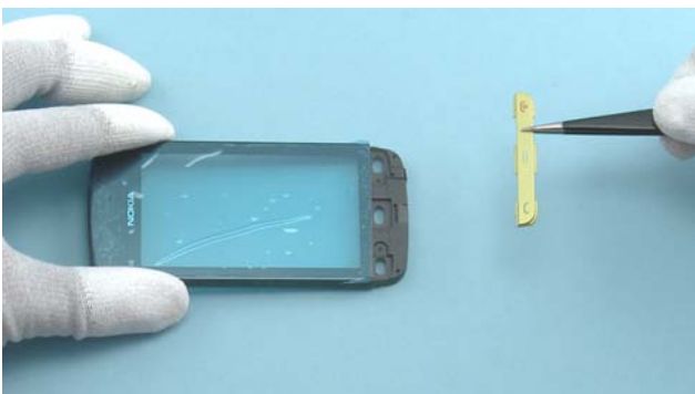
23) Remove the KEYMAT with the tweezers.
