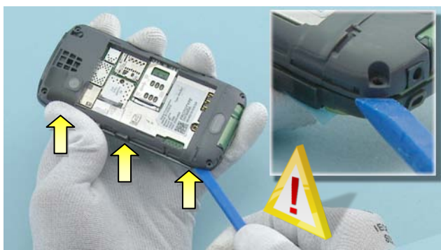
11) Use the SS-93 to detach the three shown clips of the FRONT COVER ASSEMBLY . Be careful not to damage any nearby components.
